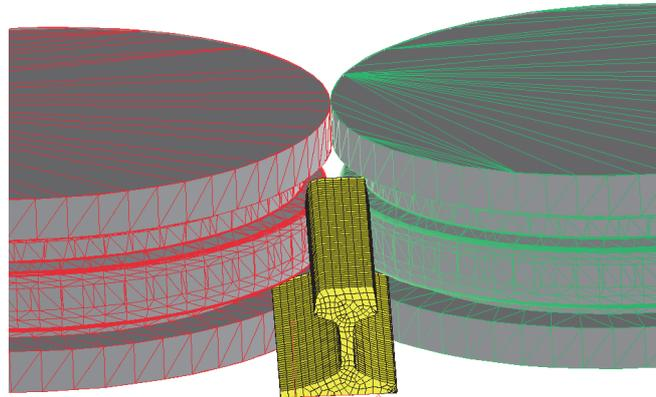
**Fig. 4** View of the roll-workpiece implemented into the Larstran-PEP software
