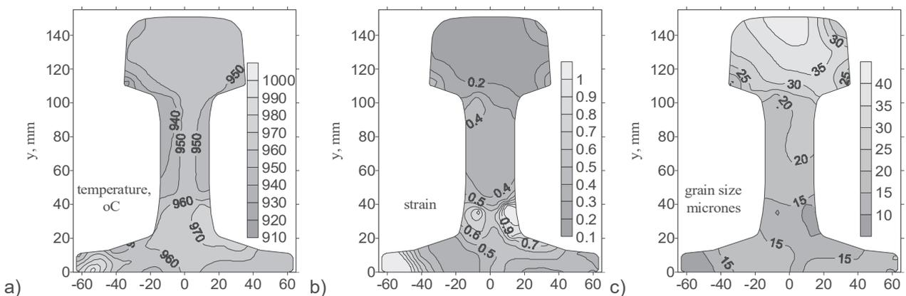
**Fig. 6** Distribution of the temperature (a); effective strain (b) and the austenite grain size (c) at the cross section of the rail after exit from the last pass
