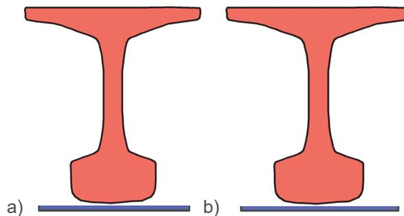
**Fig 2** Schematic illustration of one stage of controlled cooling; a) head above the level of the solution; b) head immersed in the solution.
