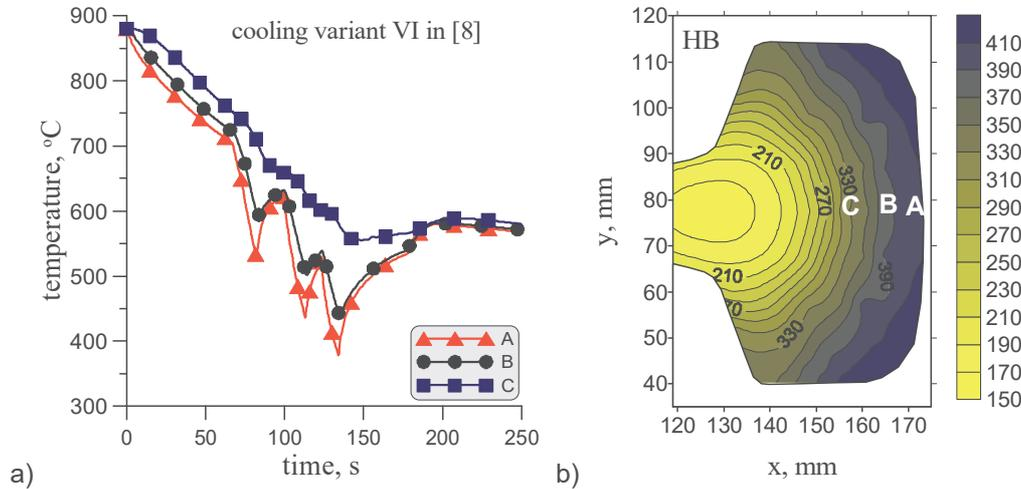
**Fig. 7** Time-temperature profiles at 3 location at the rail head (a) and hardness distribution at the cross section of the rail head (b)
