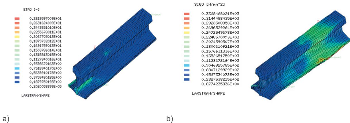
**Fig. 5** View of the rail with distribution of strains (a) and stresses (b) in the roll gap in the last pass
