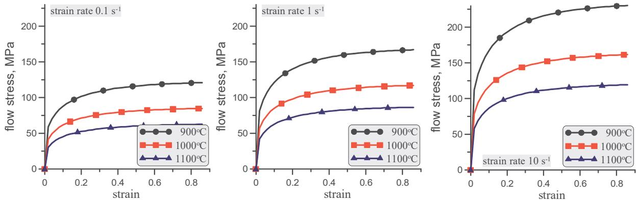
**Fig. 1** Flow stress of the investigated rail steel as a function of strain for different strain rates and temperatures.
