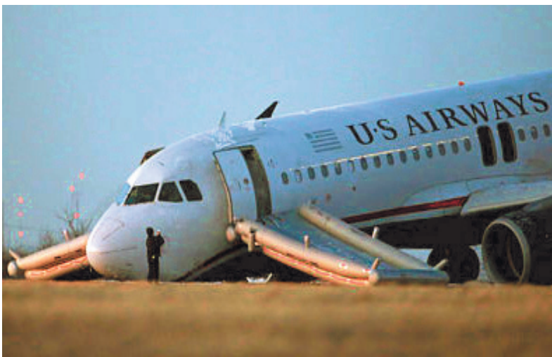
Fig. 1 Airbus A 320 crash due to break of front landing gear during take-off in March 2014. Source Novinky.cz
