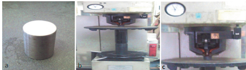
Fig. 5 View of after polishing one of hardness test specimen (a), when a hardness test was applying (a,b)
