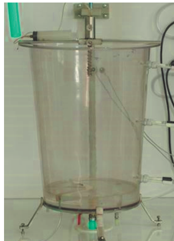
Fig. 1 Model of the ladle with top nozzle element and bottom stir element in a scale 1 : 9
