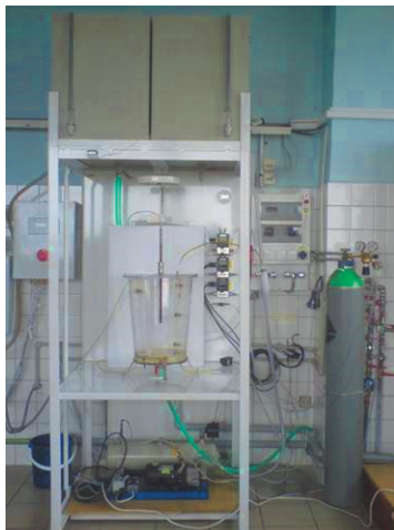
Fig. 1 Model of the ladle with top nozzle element and bottom stir element in a scale 1 : 9
