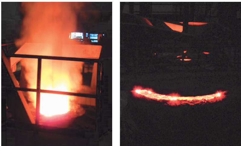
Fig. 2 Homogenisation station (HS) with the top nozzle element in the Fig. 2 where steel homogenization by the help of argon, namely by the top nozzle element ( 700 \text{ l}\cdot\text{min}^{-1} ) and bottom stir element ( 400 \text{ l}\cdot\text{min}^{-1} ) takes place. The intensive steel homogenization under the slag which has a weak desulphurization effect is a primary aim of this unit. However, conditions are the same for the whole experiment (chemical composition and slag temperature don't change significantly). Homogenization station seems to be appropriate for desulphurization study and for the subsequent verification with the results of physical modelling under the same marginal model conditions.
