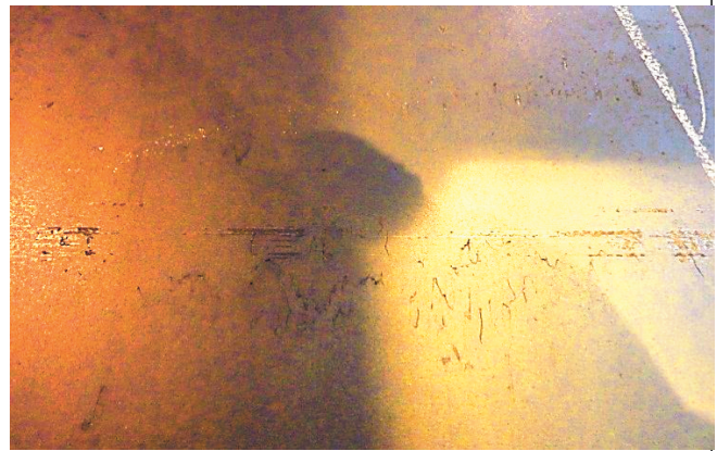
Fig. 3 Determined defects on sheets
