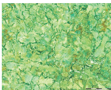
Fig. 8 LGI 2/2, Sc 0,74+0,15% AlSi, etched,100x.
