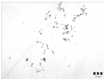
Fig. 11 Clusters of non-metallic particles, 1000x
