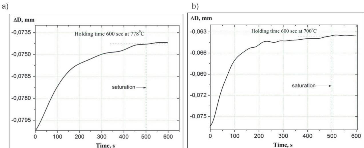
**Fig. 6** Isothermal holding of 10 min for ferrite transformation: a)  $778\text{ }^{\circ}\text{C}$ ; b)  $700\text{ }^{\circ}\text{C}$
