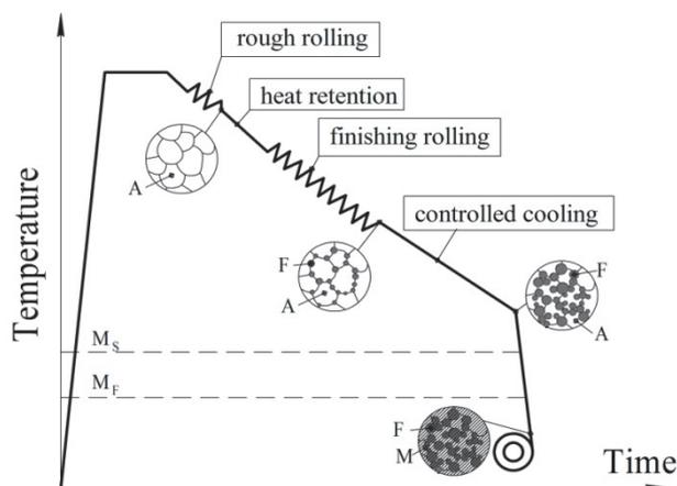
**Fig. 1** The hot rolled DP-steels production scheme (A - austenite; F - ferrite; M - martensite;  $M_s$  - martensite start temperature;  $M_f$  - martensite finish temperature)
