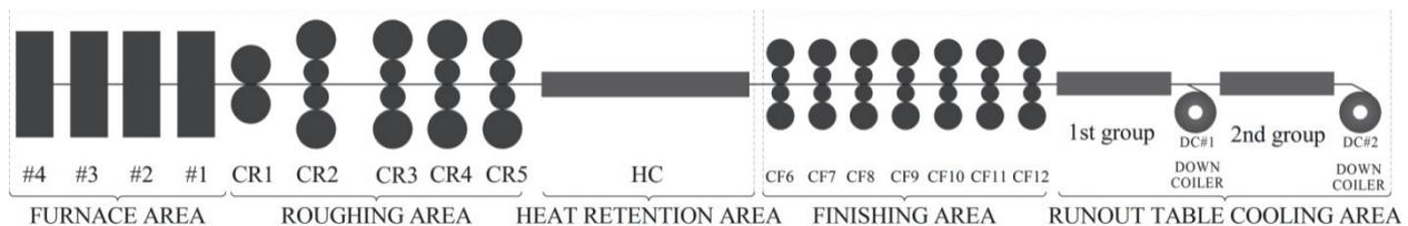
**Fig. 2** The rolling mill 2000 scheme
