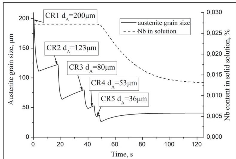
**Fig. 3** The calculation results of austenite grain size and concentration of Nb in solid solution
