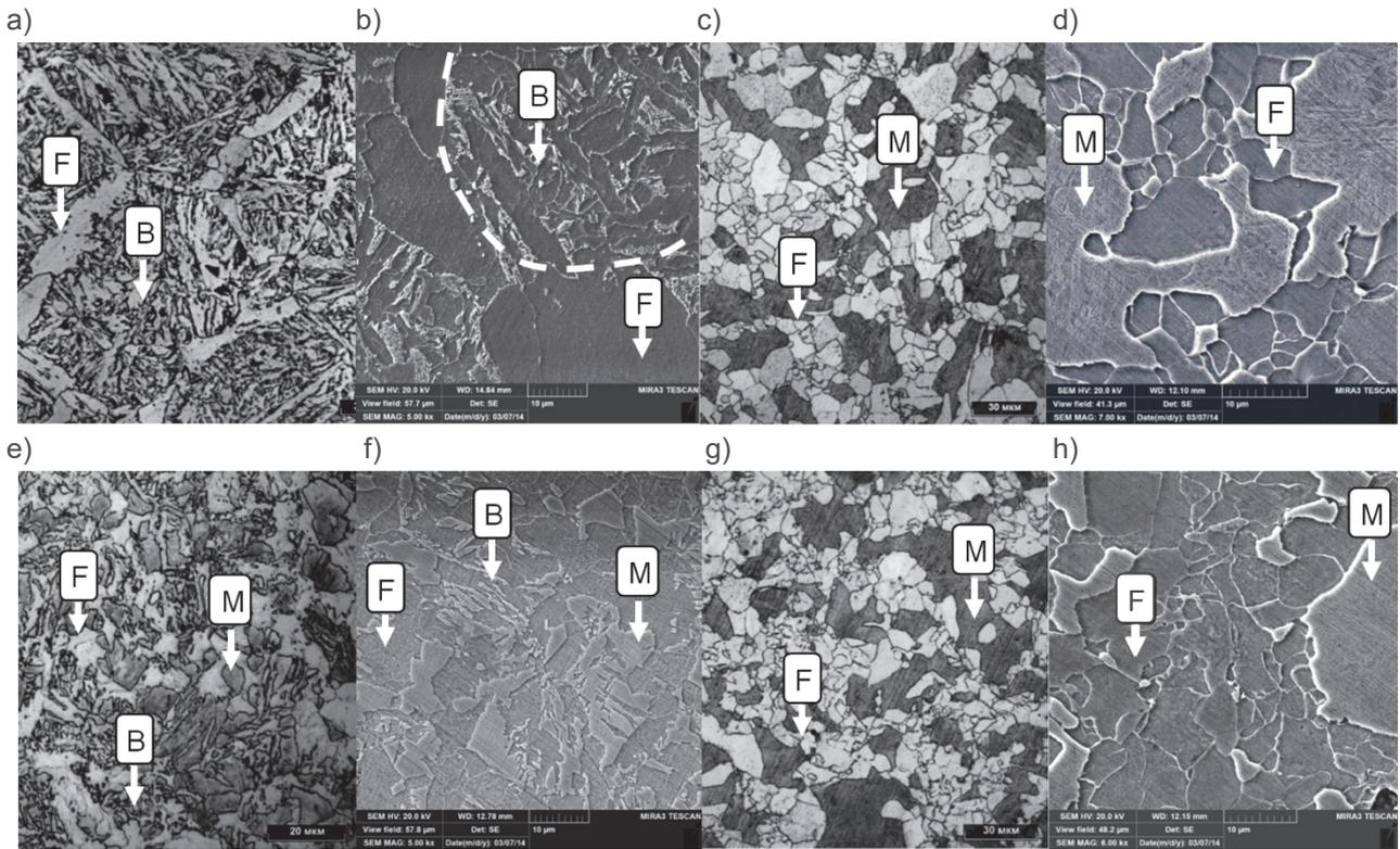
**Fig. 5** The microstructures received after physical simulation according to schedules: a), b) schedule 1 ( $\times 500$ ;  $\times 5000$ ); c), d) schedule 1a cooling rate  $15\,000\text{ }^{\circ}\text{C/s}$  ( $\times 500$ ;  $\times 7000$ ); e), f) schedule 2 ( $\times 500$ ;  $\times 5000$ ); g), h) schedule 2a cooling rate  $15\,000\text{ }^{\circ}\text{C/s}$  ( $\times 500$ ;  $\times 6000$ ); F - ferrite; B - bainite; M - martensite
