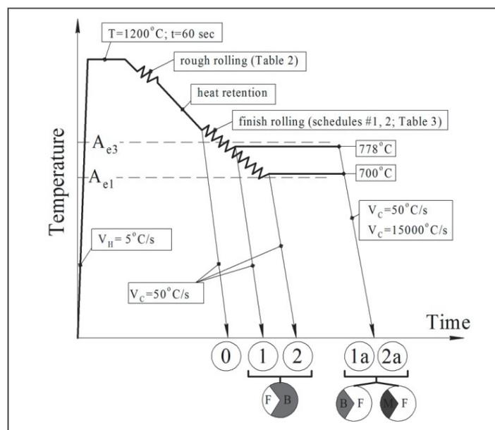
**Fig. 4** The experiments scheme realized on *Gleeble-3800*
