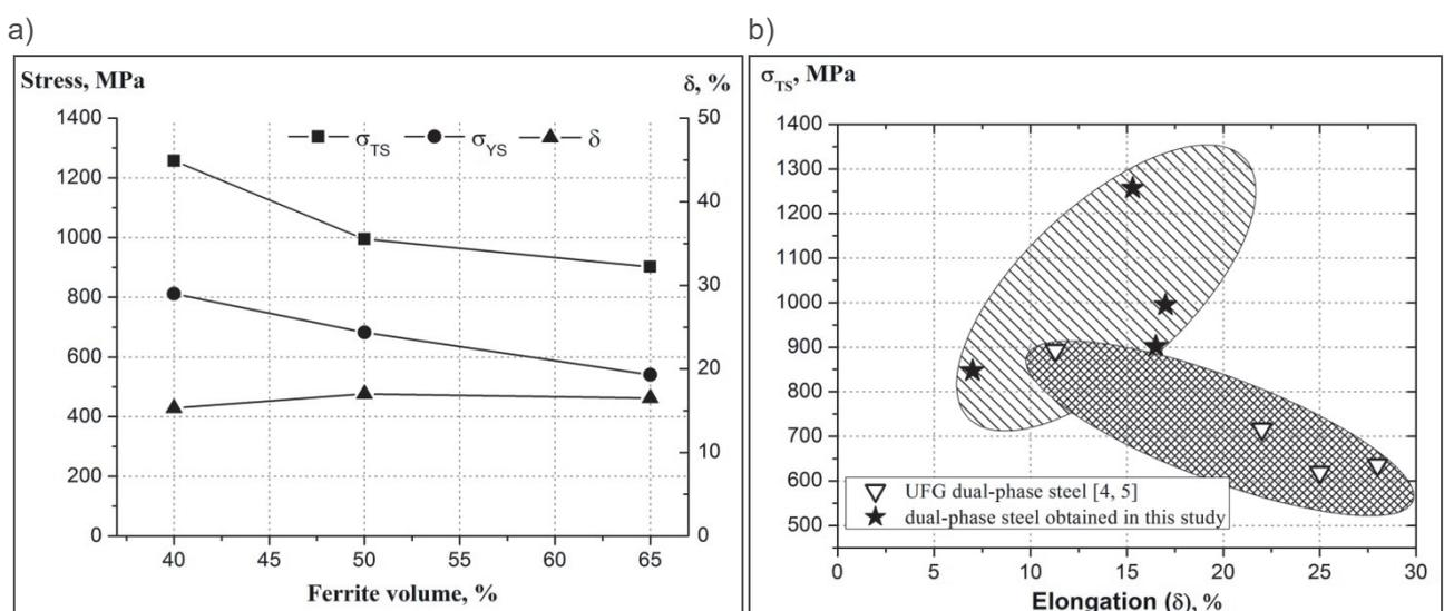
**Fig. 7** The influence of ferrite volume fraction on experimental chemical composition DP-steel properties (a); mechanical properties of received steels compare to steels received in different researches [4, 5] (b)
