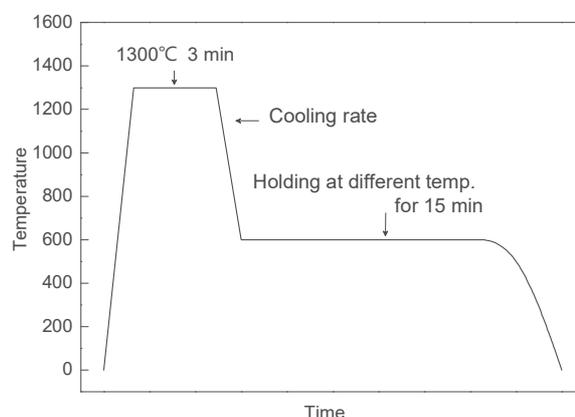
**Fig. 1** Heat treatment simulation of SS400 steel on Gleeble 1500
