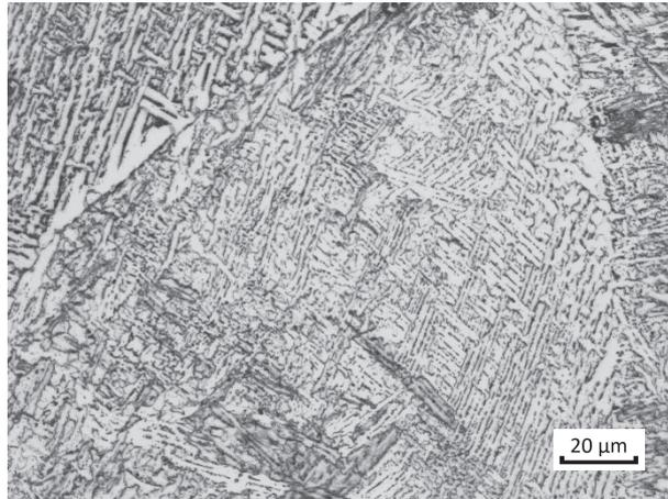
**Fig. 4** Optical micrograph showing primary microstructure of D4. The sample consists essentially of acicular ferrite with very little polygonal ferrite and bainite
