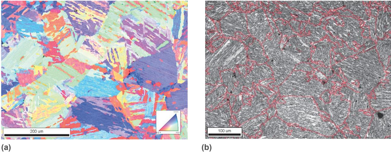
**Fig. 3** (a) IPF image of prior-austenite grain and (b) prior-austenite grain boundary
