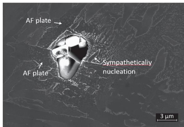
**Fig. 5** SEM morphology of acicular ferrite and MgO-spinel complex inclusion.
