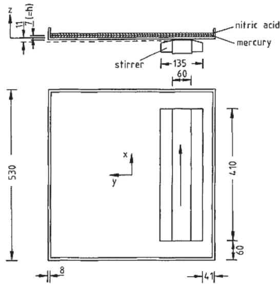
**Fig. 5** Schematic drawing of MHD experiment [9]
