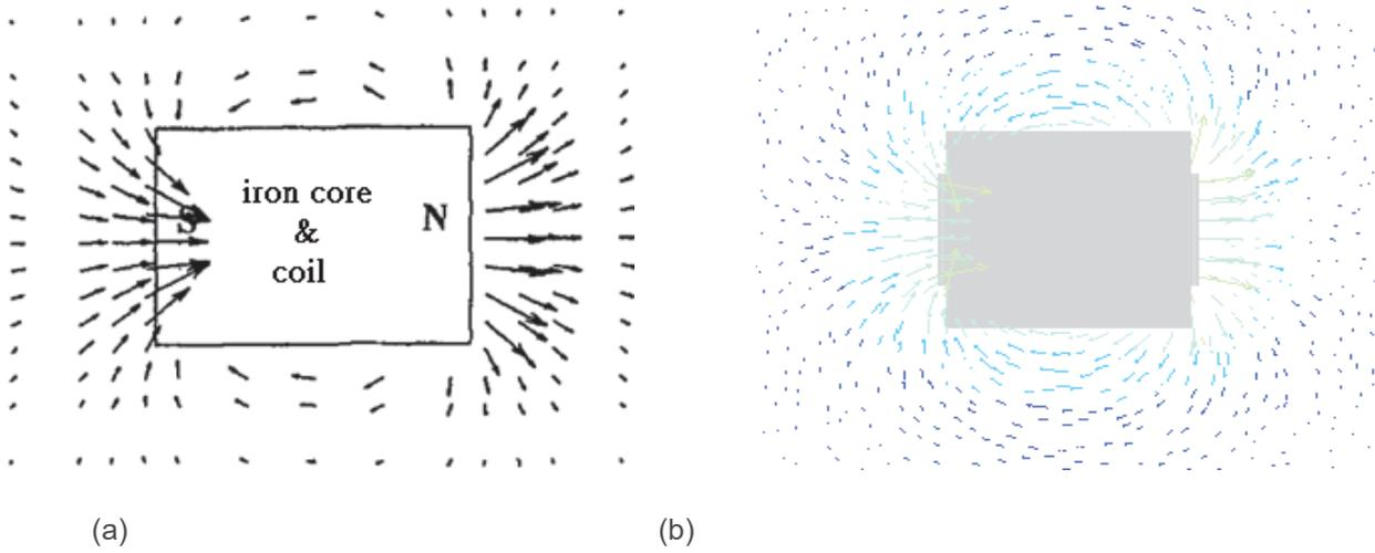
**Fig. 3** Magnetic field distribution obtained from (a) experiment [7] and (b) simulation using proposed models
