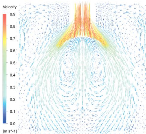
**Fig. 8** Velocity field of molten steel at  $y = 0$
