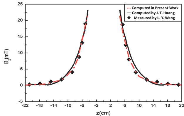
**Fig. 4** Distribution of induced magnetic density in z direction at  $x = 0$  and  $y = 0$
