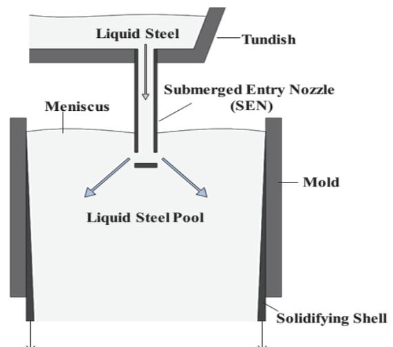
**Fig. 1** Schematic of continuous casting process
