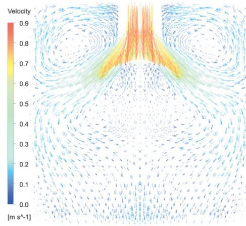
**Fig. 9** Velocity field of molten steel under effect of EMBR at  $y = 0$
