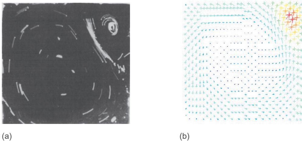
**Fig. 6** Flow pattern of mercury under effect of magnetic field from (a) measurements [9] and (b) simulation using proposed models
