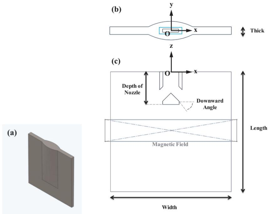
**Fig. 7** (a) Schematic of funnel-shaped mold. (b) Top view and (c) cross section of mold at  $y = 0$
