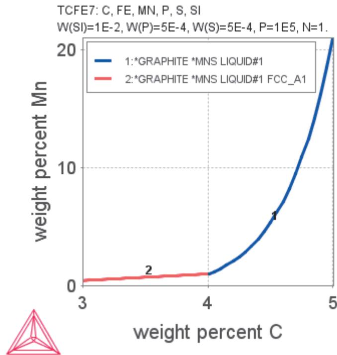
**Fig. 1** Plot of relation between content of Mn and C in Fe-C-Si-Mn-S-P system, at which MnS and Graphite would begin to solidify simultaneously, under equilibrium conditions
