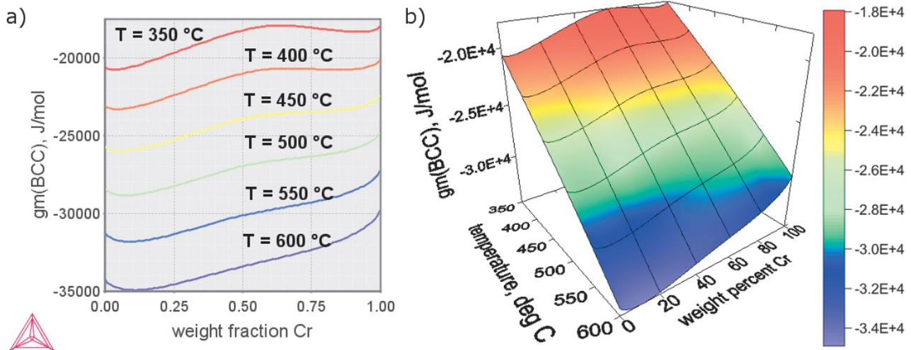
**Fig. 4** Dependency of Gibbs Free Energy of BCC phase on wt. % Cr and temperature in Fe-Cr system
