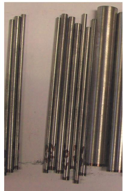
**Fig. 3** Sticks with different diameter for all three thermo analytical methods
