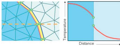
**Fig.3** Illustration of the coincident interface between two different domains [15]
