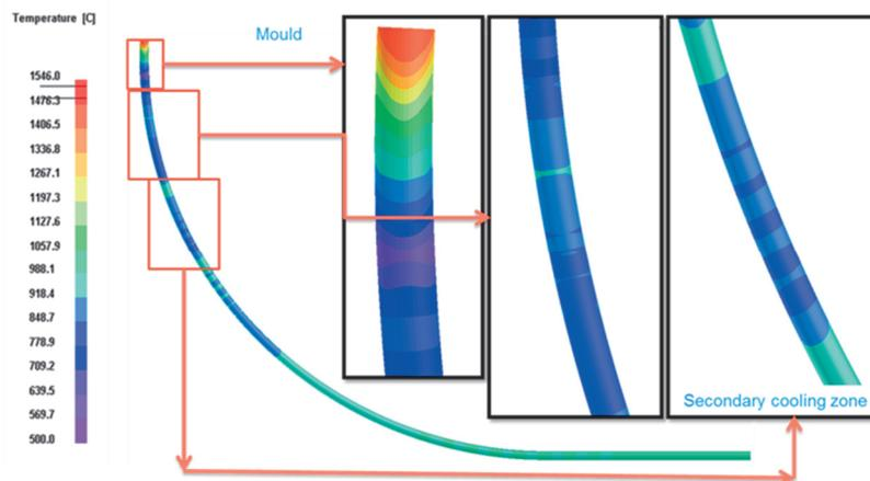
**Fig. 4** Temperature field on the surface of the strand
