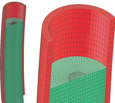
**Fig. 2** Detailed view of the computational mesh in the mould and strand area
