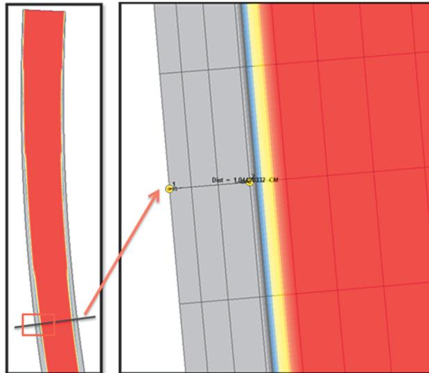
**Fig. 5** Thickness of solidified shell at the end of the mould, which was 10.4 mm
