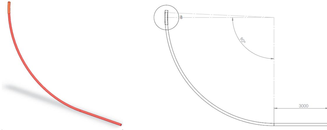
**Fig. 1** Geometry of the round format CCM with a diameter of 130 mm specified for the computation
