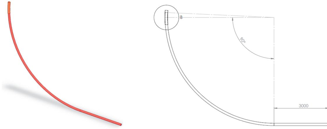
**Fig. 1** Geometry of the round format CCM with a diameter of 130 mm specified for the computation
