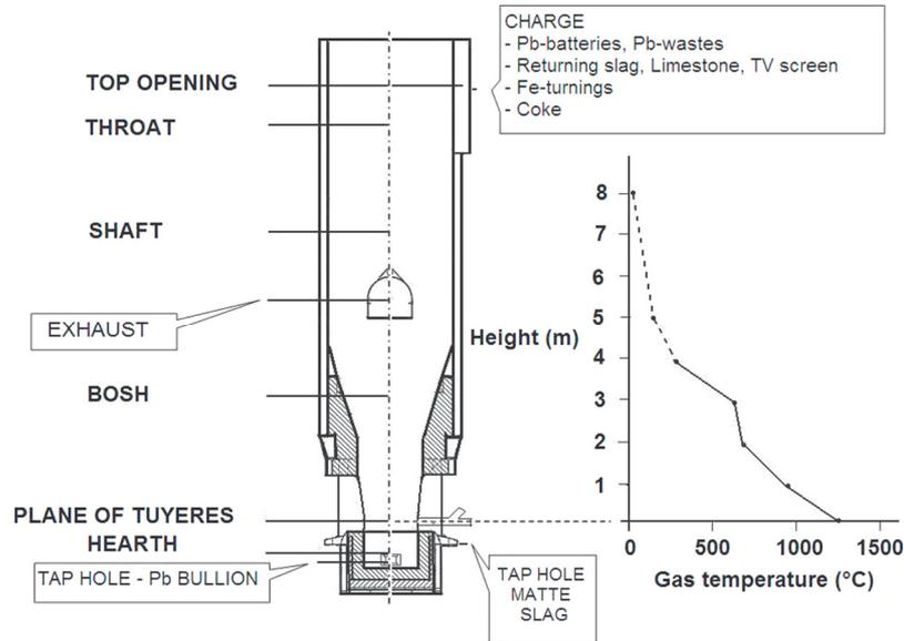
Fig. 1 Scheme of blast furnace for lead recycling, Kovohute Pribram
