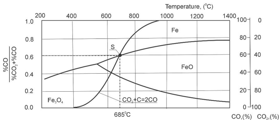
**Fig. 2** Equilibrium of iron oxides with Boudouard reaction
