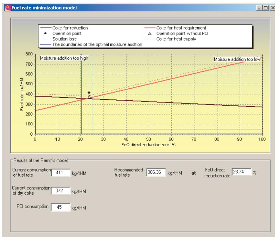
Fig. 5 Example of simulation when blast furnace operates with the ULCOS technology.
