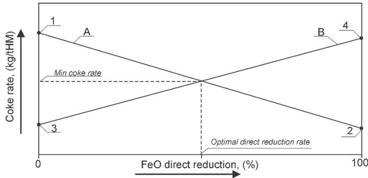
**Fig. 1** The structure of Ramm’s principles.
