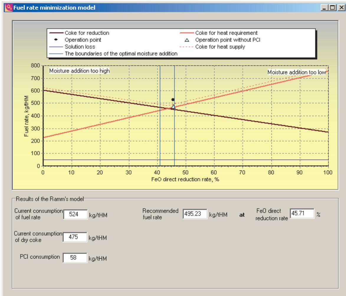
**Fig. 3** Appearance of the fuel rate minimization model
