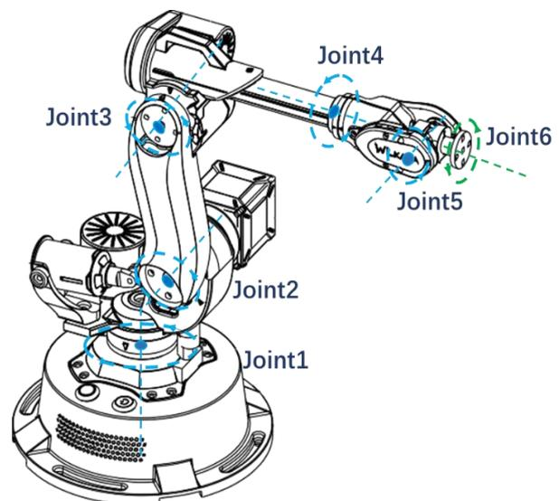
**Figure 3** Joints on WLKATA MIROBOT
