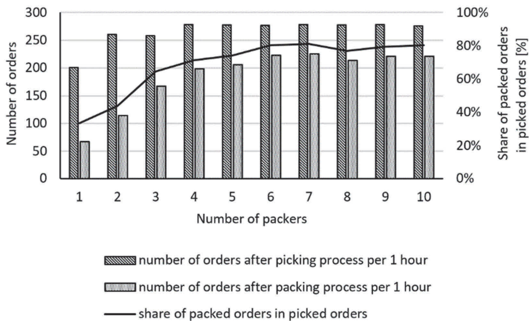
Figure 6 Efficiency of packing stations with the use of different number of packers
