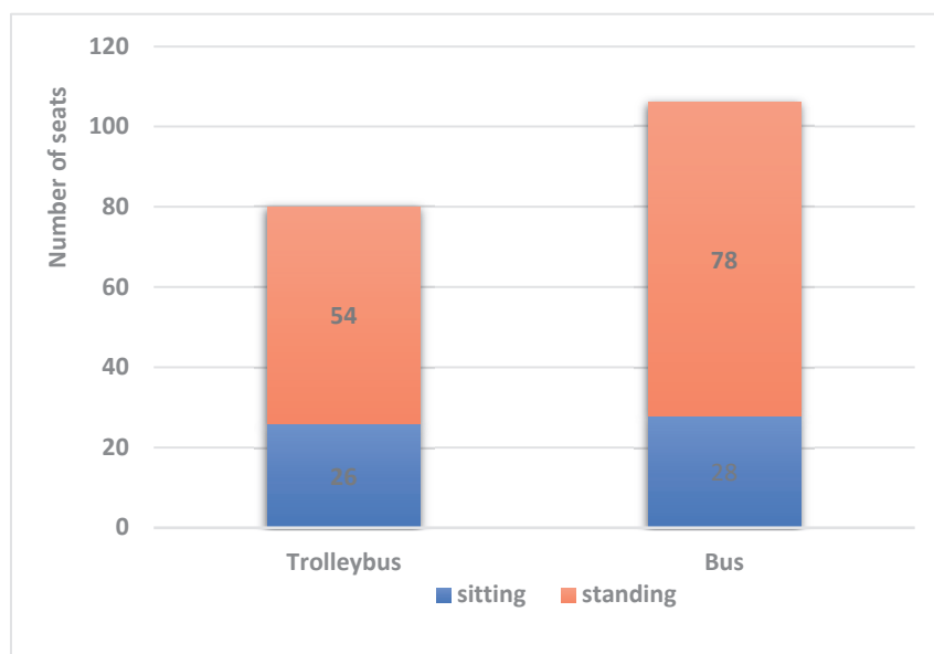
Diagram 1 Comparison of the passenger capacity of Škoda 26 Tr Solaris trolleybus and Solaris Urbino 12 CNG bus
