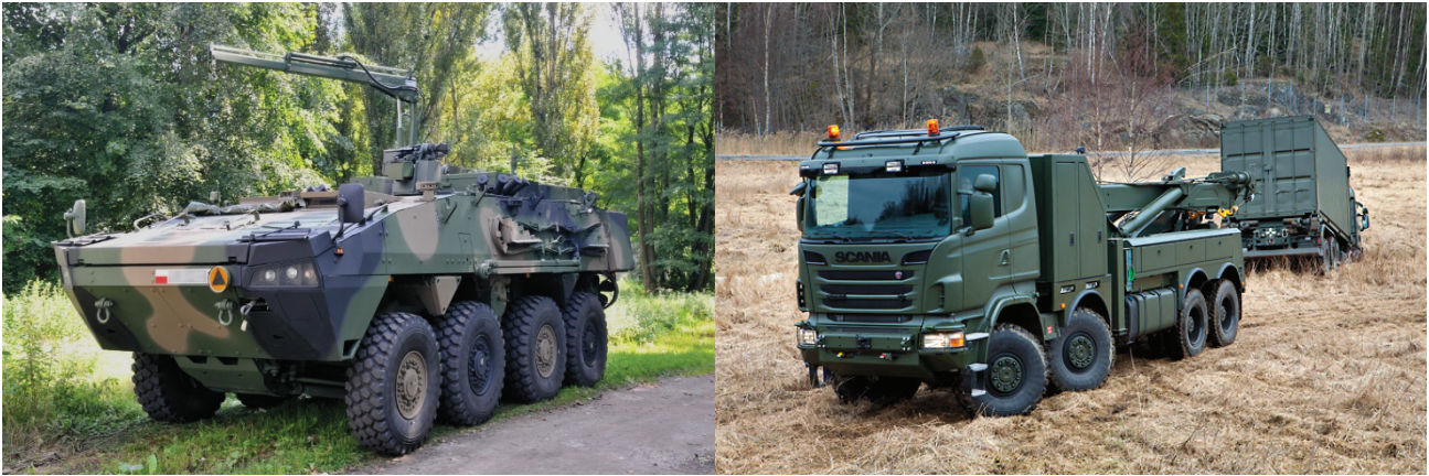
Figure 2 Wheeled vehicles for technical reconnaissance and evacuation. On the left - technical reconnaissance vehicle ROSOMAK WRT [7], on the right - technical evacuation vehicle SCANIA R 730 [8]
