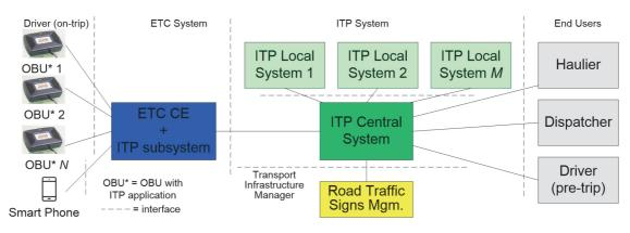
Figure 7 Structure of the system proposal
