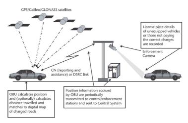
Figure 1 Principle of a satellite system [9]
