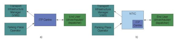
Figure 4 Logical architecture of a) dedicated ITP system and b) ITP system incorporated in the framework of NTIC - an example for information and reservation service
