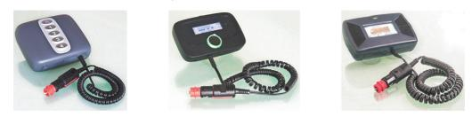
Figure 5 OBUs used in the Slovak electronic toll collect system
