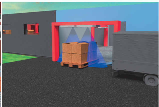
Figure 6 Reading the pallet in warehouse exit
