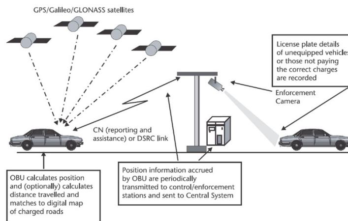
**Figure 1** Principle of a satellite system [9]
