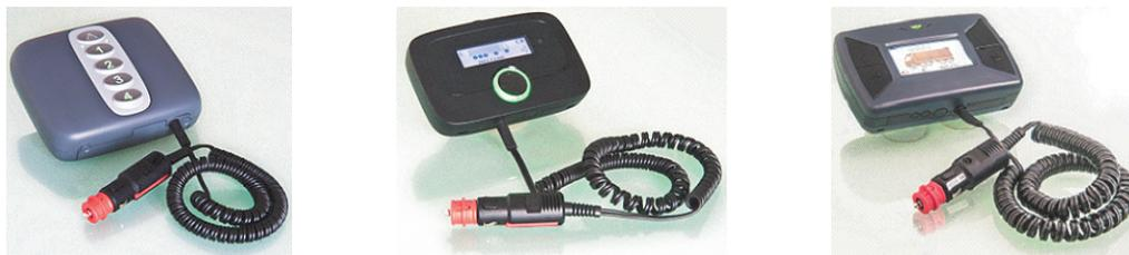
**Figure 5** OBUs used in the Slovak electronic toll collect system
