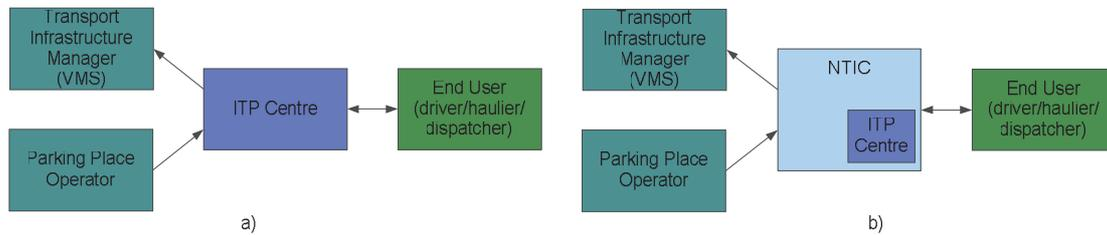
**Figure 4** Logical architecture of a) dedicated ITP system and b) ITP system incorporated in the framework of NTIC - an example for information and reservation service
