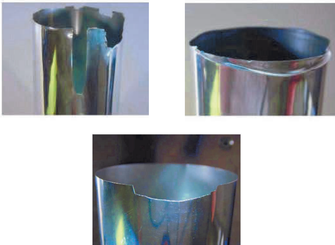
Figure 5 Examples of defects that are classified as 'short cans' (Source: Own elaboration)
