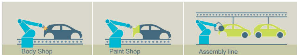
Figure 1 Stages of the production line [9]
