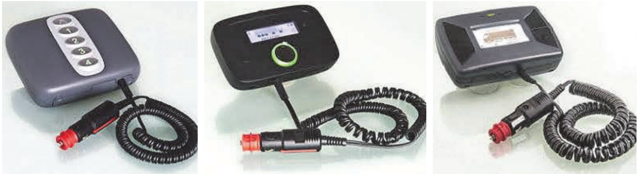
Figure 3 OBU used in the Slovak electronic toll collect system
