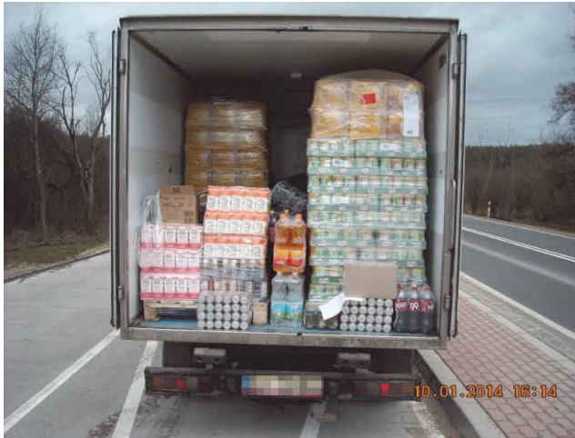
Figure 3 View of load box overloaded delivery vehicle with homogeneous cargo without the lift gate [14].
