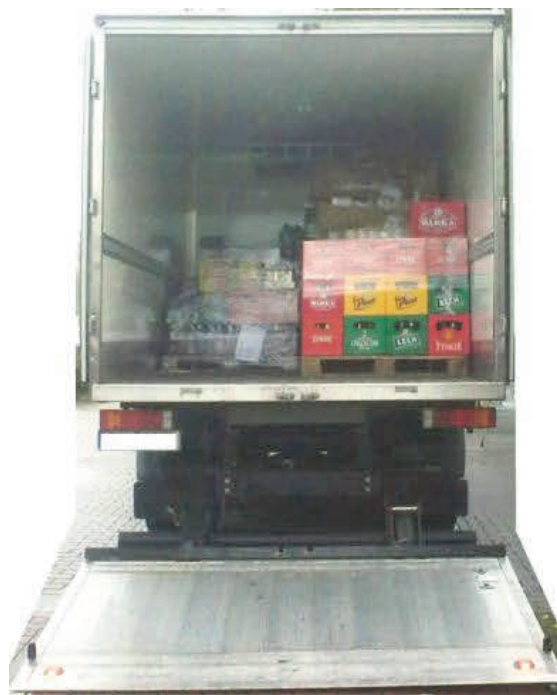
Figure 2 Delivery truck equipment with a lift gate with packages of cargo on pallets for each recipient (Own work).
