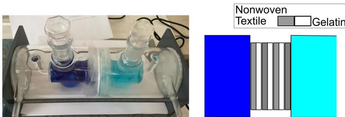
**Figure 1** Measurement of the diffusion coefficient on side-by-side cells with a membrane consisting of 8 layers of non-woven fabric connected by 3% (w/w) gelatine hydrogel after 8 hours
