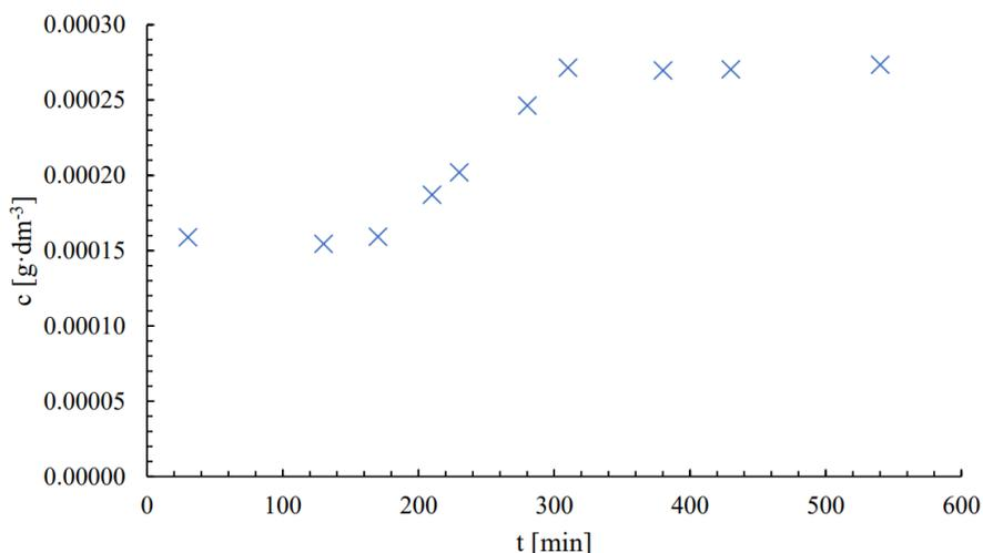
**Figure 2** Dependence of the concentration of methylene blue released from the 8-layered material on time
