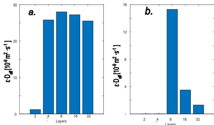
**Figure 4** Effective diffusion coefficients for various layered materials: a. Derived from the first linear segment of the material. b. Derived from the second linear region (the second linear region was not observed in the materials with 2 and 4 layers, as shown in Figure b)
