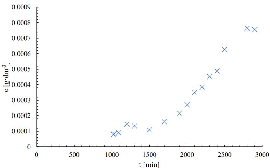
**Figure 3** Dependence of the concentration of methylene blue released from the 32-layered material on time
